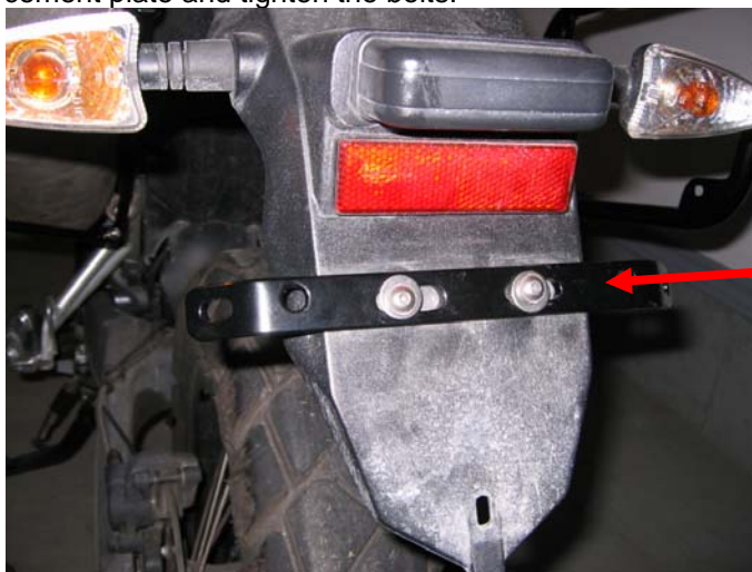
Mud flap reinforcement plate. Use M6x15 panheads and large washers
